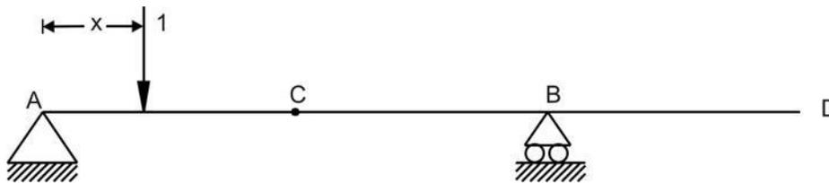
**Figure 1: A unit load before section C**
